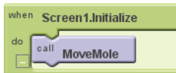
Figure 14-8. Using a Screen1.Initialize event block to move the mole when the app begins
